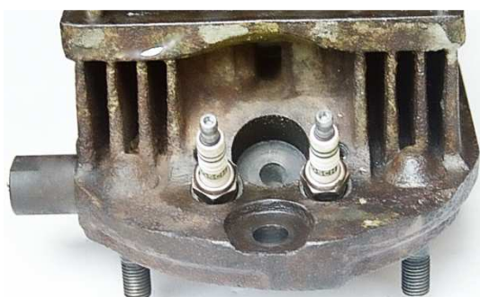
FIG. 2 Spark Plugs Location on the Cylinder Head
